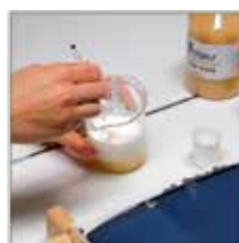
Mix the decolorant with printing paste
