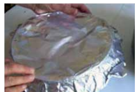
Place the protected roll of silk in the basket then cover with a sheet of aluminum foil to protect it from condensed water drops.
