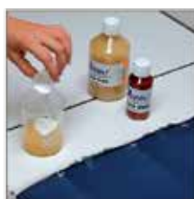
Mix the decolorant with printing paste
