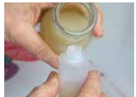
Pour the gutta into the bottle, add a few drops of solvent (essence F)
